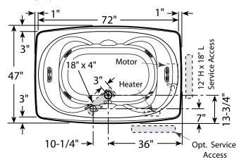
Product Shown: Sabella<sup>™</sup> Whirlpool Bath Right Hand Shown Model: EH90 \* Measurements inside unit represent cutout in floor to allow for drain/overflow. Minimum Service Access dimensions given.
